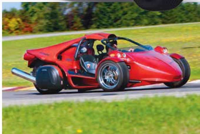
Top: The 2014 Elio by Elio Motors is an autocycle that is marketed as an efficient and practical form of transportation, with an average gas mileage of 84 mpg. Bottom: The T-REX 16S by Campagna Motors is a sporty autocycle with an in-line six-cylinder BMW engine of 1649cc.
